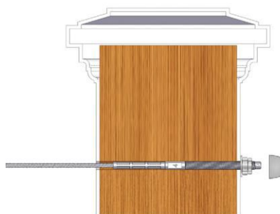
The two common types of cable railing systems include surface-mount systems (left) and through-post systems (center). Note that through-post systems will require some staggering of cable heights at corners (right).
